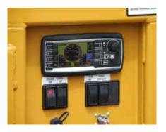
On the H-1030, the tub rotation feeds the hammermill using a Wachendorf Electronic Control Governor, which stabilizes engine load by adjusting or stopping the tub speed. It also controls tub direction, clockwise, stop, and counterclockwise as well as tracking grinding hours.
