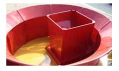
Grain grinding with a Haybuster PTO tub grinder has become a very popular use of our hay grinding machines. Installing a grain grinding hopper on the hammermill and changing screens will convert the H-1030 into a high-capacity grain grinder.
