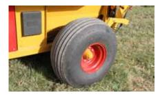
Large flotation implement tires provide for easy transportation and a stable base for the H-1030.
