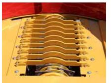
The new heavy-duty bolt-in mill grate/9 bar mill grate combination is designed to allow the operator the ability to change the number of mill grate bars and slug bars as grinding conditions change
