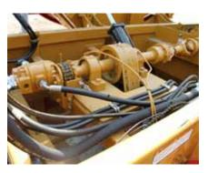
The 8 multiple belt drive system has been designed to handle increased horsepower and rotor speed. The spring tension belt drive system allows for constant belt tension while belts stretch and wear without having to manually adjust.
