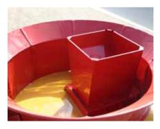
High-capacity grain grinding is another important operation that the H-1000 can also accomplish. By placing the optional grain-grinding hopper over the hammermill opening and changing screens, the H-1000 becomes a high capacity grain grinder for grinding and/or cracking feed grains.
