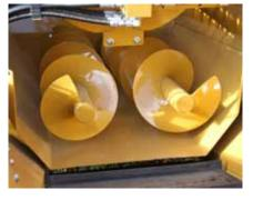
The H-1030 has 12" diameter x 4' long dual augers for discharging ground product. Augers are mounted with two heavy-duty bearings located at the base of the discharge, allowing free flow of product to the stacking conveyor. Expansion of the discharge area allows for higher capacity and reduces possibility for plugging.
