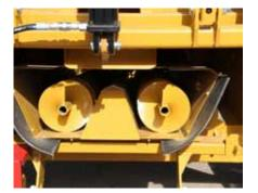
The dual 9" high-capacity augers mounted in the belly pan discharge the ground product to the stacking conveyor. The belly pan provides a clean area to catch and discharge small product such as ground corn and barley.
