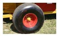
Large 16.5 x 16.1, 14-ply flotation implement tires provide for easy transportation and a solid base for the H-1130.
