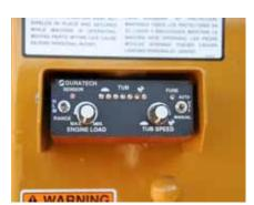
The tub rotation is controlled by an electronic governor that stabilizes engine load by adjusting the tub speed based on rotor speed. It also controls tub direction and tub stop.
