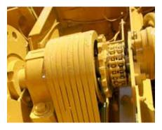
The belt drive system for the hammermill has 8-5 VP belts to handle the increased rotor speed and increased horsepower capacity. The spring tension belt drive automatically adjusts belt tension as the belts stretch.
