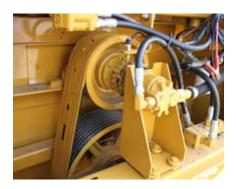
The 8-groove belt system delivers sufficient power from the PTO to the hammermill. The system has a fixed belt tension to accommodate, stretch and wear without having to monitor belt tension. This drive system turns the mill at approximately 2 x PTO speed. This mill speed provides for smooth feeding and delivers high capacity grinding performance.
