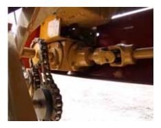
The hydraulic folding stacking conveyor is powered by a positive mechanical drive system.
