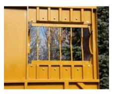
The heavy-duty bolt-in mill grate/slug bar combination is designed to allow the operator the ability to change the number of mill grate bars and slug bars as grinding conditions change. A geyser plate can be added to prevent product from being tossed straight up and out of the tub.
