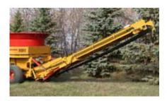
The 21' long x 24" wide hydraulically-folding conveyor is designed for the increased capacity of a 10' tub grinder. The conveoyor folds over the top of the tub for easy transport. It is capable of stacking material up to 14' 9" high at a the maximum angle.
