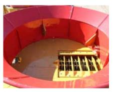
The H-1000 tub 10' 3" wide and 44 ½" deep and is constructed of a 10-gauge steel floor and a 14-gauge steel side wall. The H-1000 tub has the capacity to handle all types and sizes of bales.
