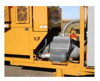
A soft start panel provides for "soft" startup for the main drive 300 hp (23.8 kw) motor. The 10 hp (7.46 kw) motor that drives the hydraulics is a direct line start. Electric motors are available in 460 volt-60 Hz, 380 volt-50 Hz, 380 volt-60 Hz and 575 volt-60 Hz. All require three phase power. Please check with your power supplier for the proper power requirements for your area before ordering.
