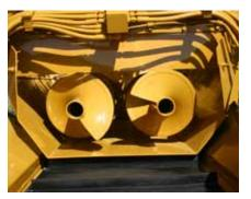
The dual 12" belly augers are suspended by two heavy-duty bearings and are located at the base of the newly-designed screen area. The auger system allows for a sealed under-screen discharge area. The larger discharge area also provides for higher capacities and reduces the potential for plugging.
