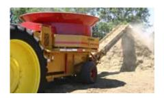
The large H-1130 Big Bite Tub is constructed of a 10-gauge steel floor and a 12-gauge steel side wall. The width of the tub is 11' 3", is 50" deep and can handle the largest round and square bales.
