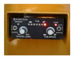
The DuraTech electronic governor slows protection for the tractor and the machine. This governor maintains a constant load on the tractor and driveline by adjusting the tubs rpm which controls the feed rate of the material to the hammermill.
