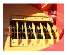
The hammermill is constructed of 3/16" thick x 15 ¾" diameter plates with 15/16" case hardened rods that hold 64-3/8" hammers. These hammers can be rotated and flipped for many hours of grinding.
